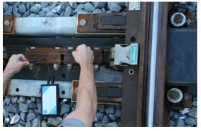
Different kinds of insulation tests can be made by connecting measurement cables to the additional test jacks.
